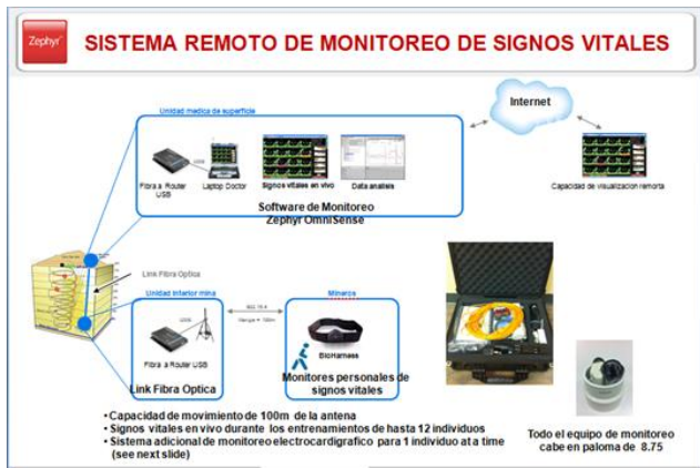
Figure 3. System for remote vital sign monitoring
